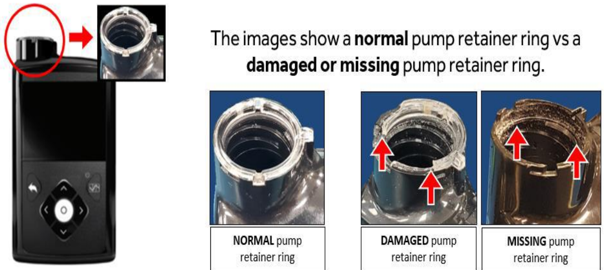
Image: Location of the retainer ring on the MiniMed™ 600 series insulin pump
